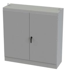
Saginaw enclosure, NEMA 3R/12/13, 72 x 72 x 24in (HxWxD), freestanding, dual access, carbon steel, ANSI 61 gray, powder coat finish, overlapping double-door, 3-point keylocking/padlocking combo handle.
