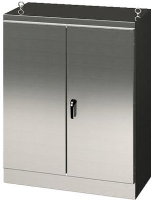
Saginaw enclosure, NEMA 3R/12/13, 72 x 72 x 18in (HxWxD), freestanding, 304 stainless steel, #4 brush finish, double-door, 3-point keylocking/padlocking combo handle.
