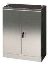
Saginaw enclosure, NEMA 3R/12/13, 72 x 72 x 18in (HxWxD), freestanding, 304 stainless steel, #4 brush finish, double-door, 3-point keylocking/padlocking combo handle.
