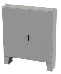
Saginaw enclosure, NEMA 3R/12/13, 72 x 72 x 16in (HxWxD), floor mount, carbon steel, ANSI 61 gray, powder coat finish, double-door, 3-point keylocking/padlocking combo handle.
