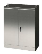
Saginaw enclosure, NEMA 3R/12/13, 72 x 60 x 36in (HxWxD), freestanding, 304 stainless steel, #4 brush finish, double-door, 3-point keylocking/padlocking combo handle.
