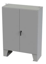
Saginaw enclosure, NEMA 3R/12/13, 72 x 60 x 24in (HxWxD), floor mount, carbon steel, ANSI 61 gray, powder coat finish, double-door, 3-point keylocking/padlocking combo handle.
