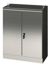
Saginaw enclosure, NEMA 3R/12/13, 72 x 60 x 24in (HxWxD), freestanding, 304 stainless steel, #4 brush finish, double-door, 3-point keylocking/padlocking combo handle.
