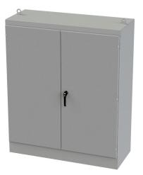
Saginaw enclosure, NEMA 3R/12/13, 72 x 60 x 24in (HxWxD), freestanding, carbon steel, ANSI 61 gray, powder coat finish, double-door, 3-point keylocking/padlocking combo handle.
