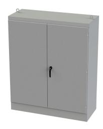
Saginaw enclosure, NEMA 3R/12/13, 72 x 60 x 24in (HxWxD), freestanding, dual access, carbon steel, ANSI 61 gray, powder coat finish, overlapping double-door, 3-point keylocking/padlocking combo handle.
