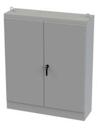
Saginaw enclosure, NEMA 3R/12/13, 72 x 60 x 18in (HxWxD), freestanding, carbon steel, ANSI 61 gray, powder coat finish, double-door, 3-point keylocking/padlocking combo handle.
