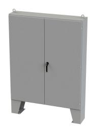
Saginaw enclosure, NEMA 3R/12/13, 72 x 60 x 12in (HxWxD), floor mount, carbon steel, ANSI 61 gray, powder coat finish, double-door, 3-point keylocking/padlocking combo handle.
