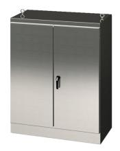
Saginaw enclosure, NEMA 3R/12/13, 72 x 48 x 24in (HxWxD), freestanding, 304 stainless steel, #4 brush finish, double-door, 3-point keylocking/padlocking combo handle.
