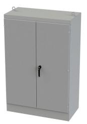
Saginaw enclosure, NEMA 3R/12/13, 72 x 48 x 24in (HxWxD), freestanding, carbon steel, ANSI 61 gray, powder coat finish, double-door, 3-point keylocking/padlocking combo handle.
