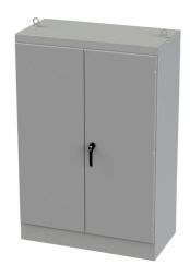
Saginaw enclosure, NEMA 3R/12/13, 72 x 48 x 24in (HxWxD), freestanding, dual access, carbon steel, ANSI 61 gray, powder coat finish, overlapping double-door, 3-point keylocking/padlocking combo handle.
