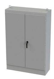
Saginaw enclosure, NEMA 3R/12/13, 72 x 48 x 18in (HxWxD), freestanding, carbon steel, ANSI 61 gray, powder coat finish, double-door, 3-point keylocking/padlocking combo handle.
