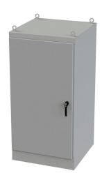
Saginaw enclosure, NEMA 3R/12/13, 72 x 36 x 36in (HxWxD), freestanding, carbon steel, ANSI 61 gray, powder coat finish, single-door, 3-point keylocking/padlocking combo handle.
