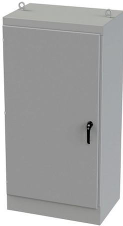
Saginaw enclosure, NEMA 3R/12/13, 72 x 36 x 24in (HxWxD), freestanding, carbon steel, ANSI 61 gray, powder coat finish, single-door, 3-point keylocking/padlocking combo handle.
