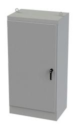
Saginaw enclosure, NEMA 3R/12/13, 72 x 36 x 24in (HxWxD), freestanding, carbon steel, ANSI 61 gray, powder coat finish, single-door, 3-point keylocking/padlocking combo handle.
