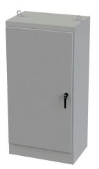
Saginaw enclosure, NEMA 3R/12/13, 72 x 36 x 24in (HxWxD), freestanding, dual access, carbon steel, ANSI 61 gray, powder coat finish, single-door, 3-point keylocking/padlocking combo handle.
