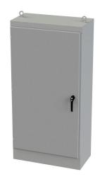
Saginaw enclosure, NEMA 3R/12/13, 72 x 36 x 18in (HxWxD), freestanding, carbon steel, ANSI 61 gray, powder coat finish, single-door, 3-point keylocking/padlocking combo handle.
