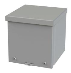
Saginaw enclosure, NEMA 3R, 6 x 6 x 6in (HxWxD), wall mount, carbon steel, ANSI 61 gray, powder coat finish, screw cover, padlock hasp and staple.
