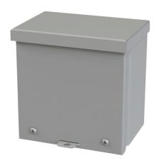
Saginaw enclosure, NEMA 3R, 6 x 6 x 4in (HxWxD), wall mount, carbon steel, ANSI 61 gray, powder coat finish, screw cover, padlock hasp and staple.
