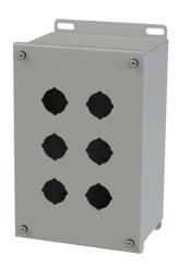
Saginaw pushbutton enclosure, 6 holes, 30mm, NEMA 4/12/13, 10 x 7 x 5in (HxWxD), wall mount, carbon steel, ANSI 61 gray, powder coat finish, screw cover.
