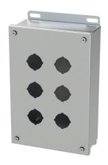
Saginaw pushbutton enclosure, 6 holes, 30mm, NEMA 4/4X/12/13, 10 x 7 x 3in (HxWxD), wall mount, 304 stainless steel, #4 brush finish, screw cover.
