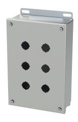
Saginaw pushbutton enclosure, 6 holes, 22mm, NEMA 4/4X/12/13, 10 x 7 x 3in (HxWxD), wall mount, 304 stainless steel, #4 brush finish, screw cover.
