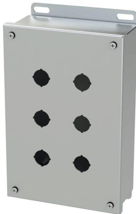
Saginaw pushbutton enclosure, 6 holes, 22mm, NEMA 4/4X/12/13, 10 x 7 x 3in (HxWxD), wall mount, 316L stainless steel, #4 brush finish, screw cover.
