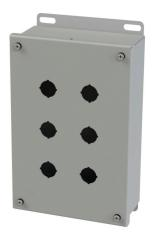
Saginaw pushbutton enclosure, 6 holes, 22mm, NEMA 4/12/13,  $10 \times 7 \times 3in$  (HxWxD), wall mount, carbon steel, ANSI 61 gray, powder coat finish, screw cover.
