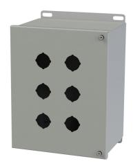
Saginaw pushbutton enclosure, 6 holes, 30mm, NEMA 4/12/13,  $10 \times 8 \times 6$ in (HxWxD), wall mount, carbon steel, ANSI 61 gray, powder coat finish, hinged screw cover.
