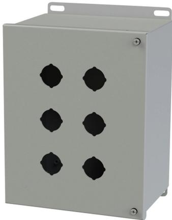
Saginaw pushbutton enclosure, 6 holes, 30mm, NEMA 4/12/13, 10 x 8 x 6in (HxWxD), wall mount, carbon steel, ANSI 61 gray, powder coat finish, hinged screw cover.
