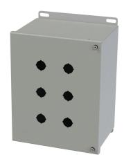
Saginaw pushbutton enclosure, 6 holes, 22mm, NEMA 4/12/13,  $10 \times 8 \times 6$  in (HxWxD), wall mount, carbon steel, ANSI 61 gray, powder coat finish, hinged screw cover.
