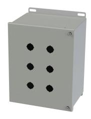
Saginaw pushbutton enclosure, 6 holes, 22mm, NEMA 4/12/13,  $10 \times 8 \times 6$  in (HxWxD), wall mount, carbon steel, ANSI 61 gray, powder coat finish, hinged screw cover.
