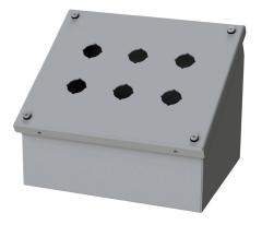
Saginaw pushbutton consolet, 6 holes, 22mm, NEMA 4/12/13, 7 x 9 x 7in (HxWxD), wall mount, carbon steel, ANSI 61 gray, powder coat finish, screw cover, purchase subpanel separately.
