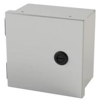
Saginaw enclosure, NEMA 1, 6 x 6 x 4in (HxWxD), wall mount, carbon steel, ANSI 61 gray, powder coat finish, single-door, 1/4-turn semi-flush latch.
