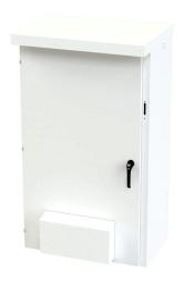
Saginaw disconnect enclosure, vented, NEMA 3R, right flange,  $65 \times 37 \times 20$  in (HxWxD), wall mount, carbon steel, white, powder coat finish, single-door, 3-point padlocking handle, purchase subpanel separately.
