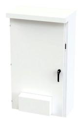
Saginaw disconnect enclosure, vented, NEMA 3R, right flange,  $65 \times 37 \times 16$  in (HxWxD), wall mount, carbon steel, white, powder coat finish, single-door, 3-point padlocking handle, purchase subpanel separately.
