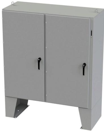
Saginaw Enviroline series disconnect enclosure, NEMA 3R/4/12/13, right flange, 60 x 61 x 24in (HxWxD), floor mount, carbon steel, ANSI 61 gray, powder coat finish, 2-door, 3-point padlocking handle, purchase subpanel separately.
