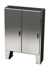
Saginaw Enviroline series disconnect enclosure, NEMA 3R/4/4X/12/13, right flange, 60 x 61 x 12in (HxWxD), floor mount, 304 stainless steel, #4 brush finish, 2-door, 3-point padlocking handle, purchase subpanel separately.
