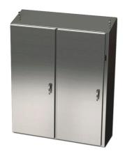
Saginaw Enviroline series disconnect enclosure, slope top, NEMA 3R/4/4X/12/13, right flange, 60 x 61 x 12in (HxWxD), freestanding, 316L stainless steel, #4 brush finish, 2-door, 3-point 304 stainless steel padlocking handle, purchase subpanel separately.
