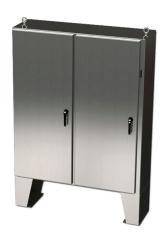
Saginaw Enviroline series disconnect enclosure, NEMA 3R/4/4X/12/13, right flange, 60 x 61 x 12in (HxWxD), floor mount, 316L stainless steel, #4 brush finish, 2-door, 3-point padlocking handle, purchase subpanel separately.
