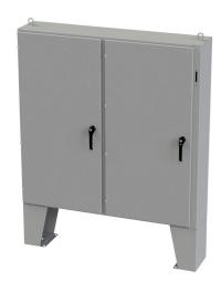
Saginaw Enviroline series disconnect enclosure, NEMA 3R/4/12/13, right flange, 60 x 61 x 12in (HxWxD), floor mount, carbon steel, ANSI 61 gray, powder coat finish, 2-door, 3-point padlocking handle, purchase subpanel separately.
