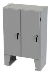
Saginaw Enviroline series disconnect enclosure, NEMA 3R/4/12/13, right flange, 60 x 49 x 24in (HxWxD), floor mount, carbon steel, ANSI 61 gray, powder coat finish, 2-door, 3-point padlocking handle, purchase subpanel separately.
