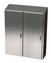
Saginaw Enviroline series disconnect enclosure, slope top, NEMA 3R/4/4X/12/13, right flange, 60 x 49 x 18in (HxWxD), freestanding, 304 stainless steel, #4 brush finish, 2-door, 3-point 304 stainless steel padlocking handle, purchase subpanel separately.
