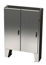
Saginaw Enviroline series disconnect enclosure, NEMA 3R/4/4X/12/13, right flange, 60 x 49 x 18in (HxWxD), floor mount, 304 stainless steel, #4 brush finish, 2-door, 3-point padlocking handle, purchase subpanel separately.
