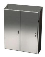
Saginaw Enviroline series disconnect enclosure, slope top, NEMA 3R/4/4X/12/13, right flange, 60 x 49 x 18in (HxWxD), freestanding, 316L stainless steel, #4 brush finish, 2-door, 3-point 304 stainless steel padlocking handle, purchase subpanel separately.
