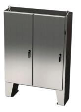
Saginaw Enviroline series disconnect enclosure, NEMA 3R/4/4X/12/13, right flange, 60 x 49 x 18in (HxWxD), floor mount, 316L stainless steel, #4 brush finish, 2-door, 3-point padlocking handle, purchase subpanel separately.
