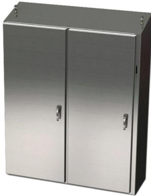
Saginaw Enviroline series disconnect enclosure, slope top, NEMA 3R/4/4X/12/13, right flange, 60 x 49 x 12in (HxWxD), freestanding, 304 stainless steel, #4 brush finish, 2-door, 3-point 304 stainless steel padlocking handle, purchase subpanel separately.
