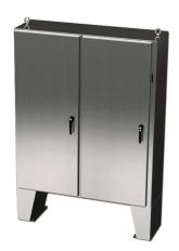
Saginaw Enviroline series disconnect enclosure, NEMA 3R/4/4X/12/13, right flange, 60 x 49 x 12in (HxWxD), floor mount, 304 stainless steel, #4 brush finish, 2-door, 3-point padlocking handle, purchase subpanel separately.
