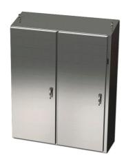
Saginaw Enviroline series disconnect enclosure, slope top, NEMA 3R/4/4X/12/13, right flange, 60 x 49 x 12in (HxWxD), freestanding, 316L stainless steel, #4 brush finish, 2-door, 3-point 304 stainless steel padlocking handle, purchase subpanel separately.
