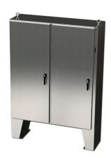
Saginaw Enviroline series disconnect enclosure, NEMA 3R/4/4X/12/13, right flange, 60 x 49 x 12in (HxWxD), floor mount, 316L stainless steel, #4 brush finish, 2-door, 3-point padlocking handle, purchase subpanel separately.
