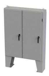
Saginaw Enviroline series disconnect enclosure, NEMA 3R/4/12/13, right flange, 60 x 49 x 12in (HxWxD), floor mount, carbon steel, ANSI 61 gray, powder coat finish, 2-door, 3-point padlocking handle, purchase subpanel separately.
