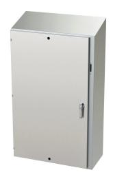
Saginaw Enviroline series disconnect enclosure, slope top, NEMA 3R/4/4X/12/13, right flange, 60 x 37 x 16in (HxWxD), wall mount, 304 stainless steel, #4 brush finish, single-door, 3-point padlocking handle, purchase subpanel separately.
