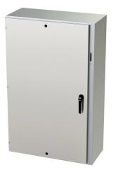
Saginaw Enviroline series disconnect enclosure, NEMA 3R/4/4X/12/13, right flange, 60 x 37 x 16in (HxWxD), wall mount, 304 stainless steel, #4 brush finish, single-door, 3-point padlocking handle, purchase subpanel separately.
