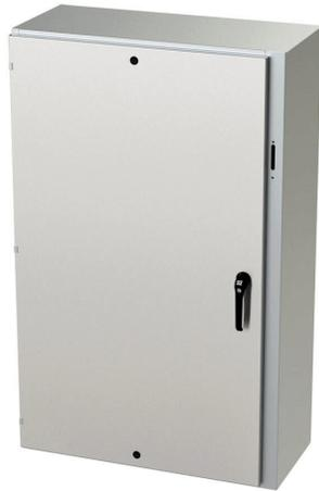
Saginaw Enviroline series disconnect enclosure, NEMA 3R/4/4X/12/13, right flange, 60 x 37 x 16in (HxWxD), wall mount, 316L stainless steel, #4 brush finish, single-door, 3-point padlocking handle, purchase subpanel separately.
