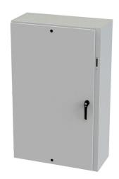
Saginaw Enviroline series disconnect enclosure, NEMA 3R/4/12/13, right flange, 60 x 37 x 16in (HxWxD), wall mount, carbon steel, RAL 7035 light gray, powder coat finish, single-door, 3-point padlocking handle, purchase subpanel separately.
